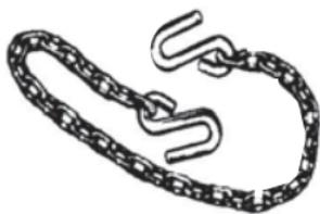
of the trailer. Make sure the hitch has provisions for the connection of **safety chains**, which are required by most states. When connected, safety chains should have some slack to permit sharp turns but should not drag on the road. In addition, they should cross under the trailer tongue to help prevent the tongue from dropping to the road in the event the trailer separates from the tow vehicle.
