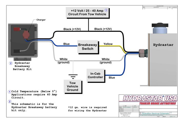
Note – The Hydrastar<sup>TM</sup> actuator does not draw power from the tow vehicle accessory lead unless the brakes on the tow vehicle are actuated.
